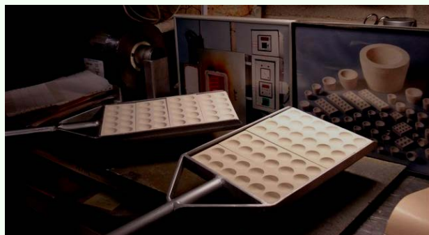
4 Bullion Block 12 HB with Fork BF 12-48 48 probes cupelled & handled in parallel
