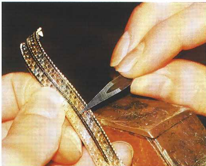
Sampling the yellow gold edging of a tricoloured bracelet
