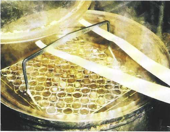
Removing the parting tray containing 96 cornets from the boiling nitric acid used to dissolve the silver
