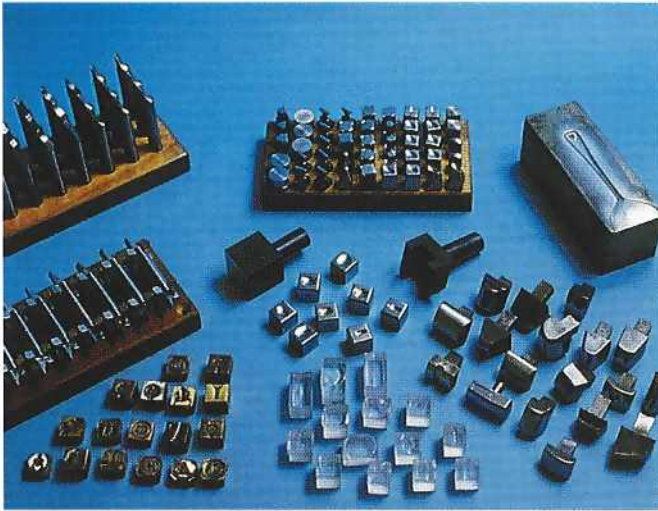
A specimen general purpose set of tools used to support jewellery and reduce damage in marking (punching)
