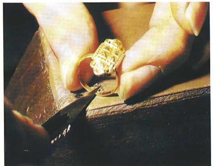
Sampling a gold ring by scraping
