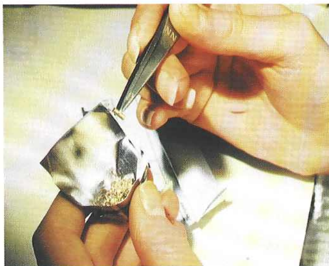
Adding silver to the weighed gold sample in its lead foil wrapper
