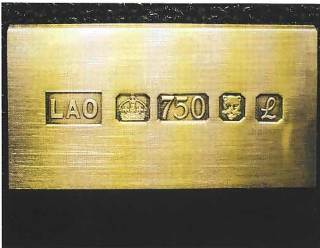
The 1985 hallmark for 750 standard gold (with London Assay Office sponsor's mark – 'LAO')
