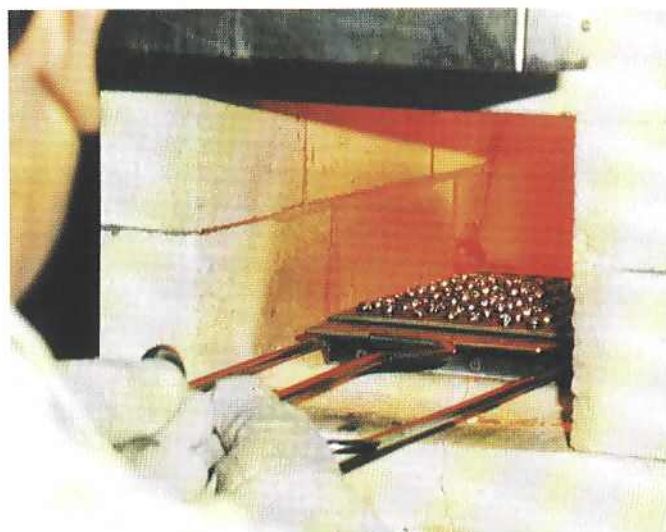
96 samples at a time are placed in preheated magnesite cupels in an electric furnace. The base metals will be extracted into the cupel
