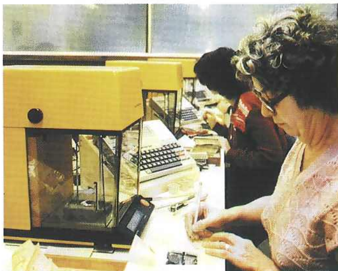
Preparing a gold sample for fire assay with the aid of computer-controlled electronic balances
