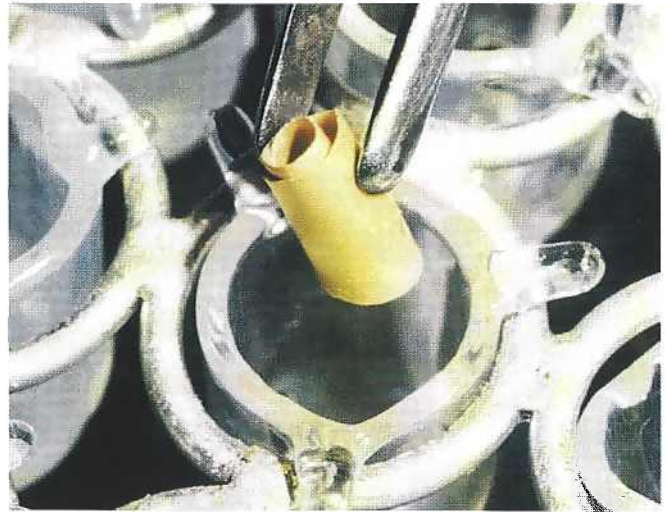
Removing one fine gold cornet from a parting thimble in readiness for reweighing
