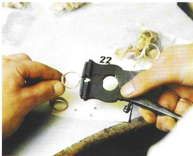
Removing the sprue from a cast ring to provide a sample for assay
