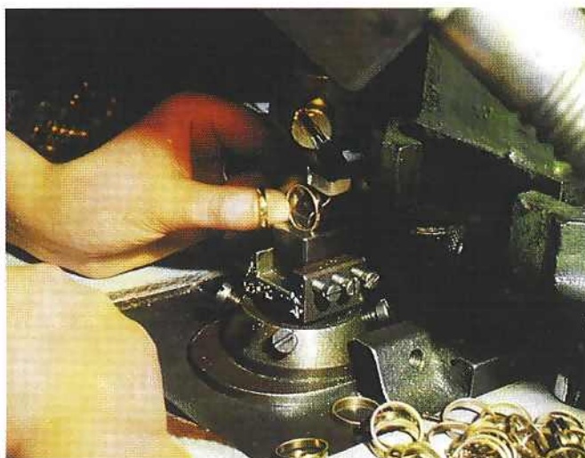
A swan-neck-shaped punch is used to apply a satisfactory mark inside a gold ring
