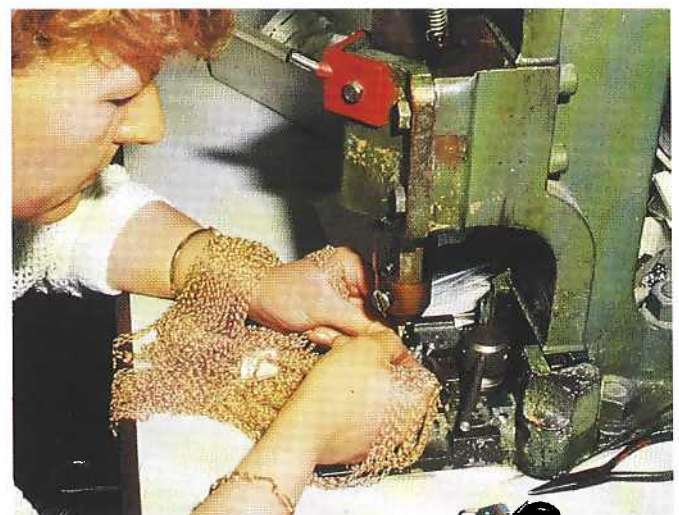
Marking gold chains on an electric reciprocating press
