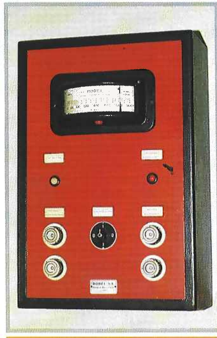
Figure 5 Temperature controller used for maintaining cupellation furnace at 1150°C
