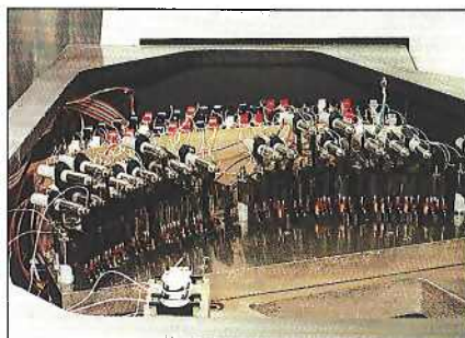
Figure 3 - Light detector in a multichannel ICP-vacuum spectrometer, Thermo-Jarrell-Ash Corp. (13)
